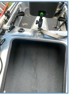
There are two scuppers that were designed for the Dragonfly transducer, one on the left and one on the right and both the most forward holes in the bottom of the kayak. I chose the left side but it doesn't matter as the rest of the install would just be on the opposite side of were it will be for this installation.
