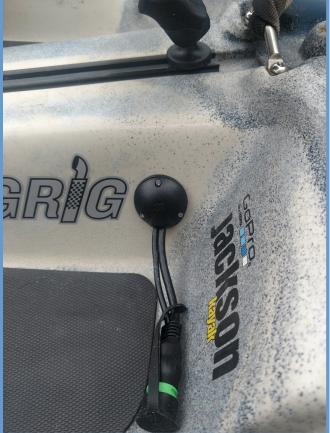
nector. After verifying this by plugging the cable in, install the bulkhead cap. This completes installation and the only task that remains is to power everything up.
