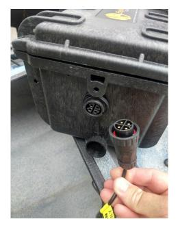
Cigarette lighter plug, recharge port, marker light, etc. are just a few examples. I'm probably going to wire those up as a charging port so as to not have to remove the battery pack from the kayak well each time. When I wire the plug for my Battery Tender charger, I will bring the wire out of the bulkhead
