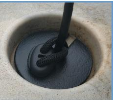
As you can see, the scupper used for mounting is just forward of the foot rest and an ideal place to drill a 1" hole to route the transducer cable into the cavity of the kayak. This will keep the cable out from under foot. (Note the unevenness of the drilled hole. I only had a 7/8" drill bit and had to file the rest out!) Now rout the cable through the drilled hole, install the Thru
